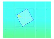
So previously the bounding-box of object "A" overlapped 16 container bins. We doubled the container bin size and now we only require 4 container bins. That sounds like a better situation doesn't it? Well yes and no.
