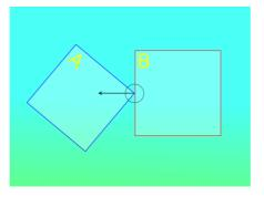
The collisions contact is a point at the centre of the black circle and the collision normal is the direction indicated by the black arrow. Note that the collision normal is pointing in the opposite direction that object "A" was moving. That's coincidence, the arrow points away from the edge of object "B" that object "A" collided with. Indeed it's always **perpendicular** to the edge. So how are these used for a collision response? Let's go through some responses starting with bounce:
