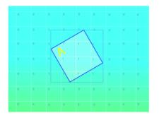
As you can see, having the object "A" in the scene requires us to add 16 references to it. The reason for 16 is that the bounding-box of object "A" covers 16 container bins. If we increased the size of the object we'd cover more container bins. So the penalty is that as the objects get bigger, the cost of keeping them in the scene-container rises. Thankfully though the cost is relatively small but it can easily add up with lots of objects.
