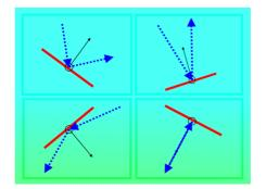
The common feature of all these bounce responses is that the incoming velocity is reflected around the collision normal. Imagine that you put a mirror along the collision normal (black line). If you looked at the pre-collision velocity you'd see it reflected as the post-collision velocity. The incoming angle of velocity is equal to the outgoing angle of velocity.
