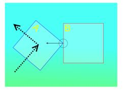
This diagram shows the direction of object "A" before it collides with object "B" as shown by the black arrow pointing up/right. After collision the "bounce" response was applied and the new direction of object "A" is shown by the second black arrow pointing up/left.
