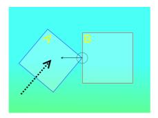
After the previous two responses this one should be easy to understand. Notice that the post-collision velocity is zero (the object has stopped). The stop collision response doesn't really need the collision normal as it just sets the velocity to zero. It's pretty easy to understand and implement. Because the stop collision response causes the object to seemingly stick to the other object (it stops in contact with it) it's sometimes known as the sticky collision response.
