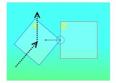
This diagram shows the direction of object "A" before it collides with object "B" as shown by the black arrow pointing up/right. After collision the "clamp" response was applied and the new direction of object "A" is shown by the second black arrow pointing up.
